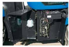
Reach batteries, washer fluid and axle lube filter through this handy right-hand service door. Steps on the door let you use a service-access window to reach the electrical components in the cab and easily route monitor cables.
